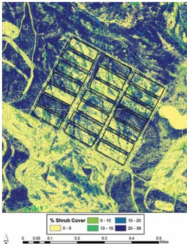
*The EST method of interpreting satellite imagery was validated against field data from an independent study of sagebrush removal. The study test plots can be clearly seen in this Ikonos satellite image. Comparison of the Ikonos cover classification with field data showed an 85% agreement. Image courtesy of Open Range Consulting.*
