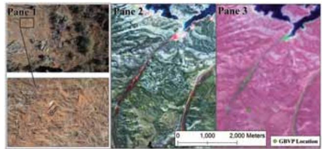
*Very high-resolution DSLR photo plots taken in the field are used to “train” geospatial models to better interpret images from Ikonos and Landsat satellite imagery. This technique delivers accurate land cover information at different scales. In Pane 1, DSLR photo plots capture cover at 2mm resolution with very fine detail; Pane 2 shows 1m-resolution Ikonos imagery; and Pane 3 shows 30m-resolution Landsat imagery. Image from Sant et al., 2014.*
